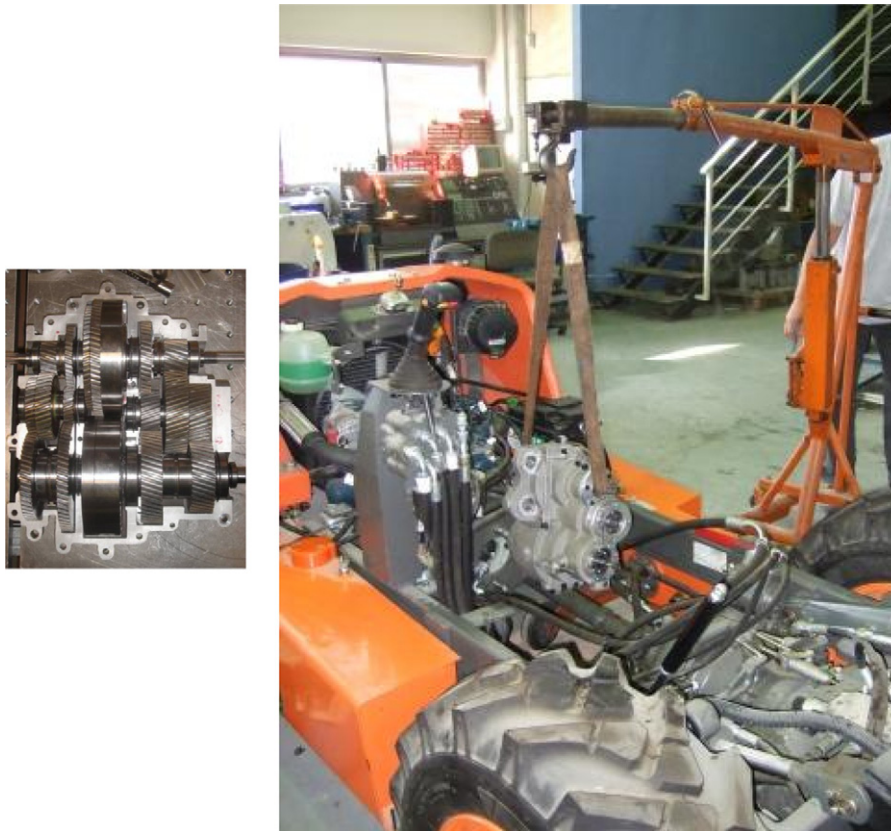
Fig. 22. The CVT transmission designed to fit in a forklift.
